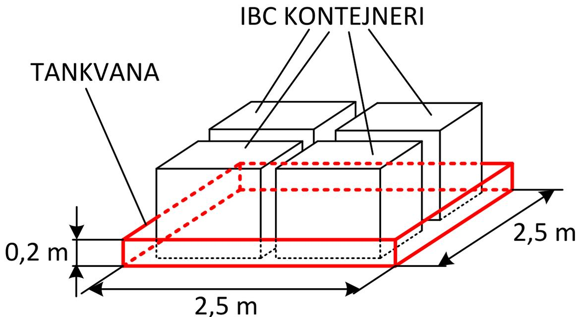
UKUPNI VOLUMEN TANKVANE:  $V_{\text{tankvane}} = 2,50 \times 2,50 \times 0,20 = 1,25 \text{ m}^3$
